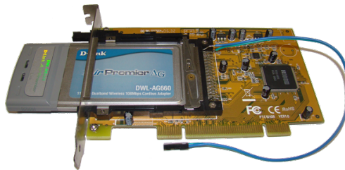
Fig. 4: NITOS PCMCIA prototype adapter for energy consumption measurements.
